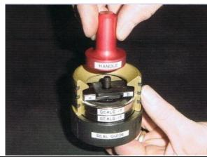
Step 4 – Screw handle onto jaw A stud until tight.
