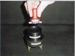
Step 4 – Place handle with A&B jaws, into counter bore on install sleeve.
