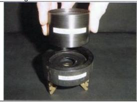
Step 3 – Place install sleeve, with counter bore facing up, on top of inserts in seal guide.
