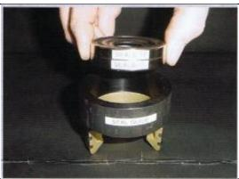
Step 2 – Place new seal inserts into seal guide, open end of insert cup, facing up on bottom seal, and the open end of cup facing down on the top seal.
