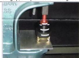
Step 5 – In a small press, with the axle seal housing on a flat surface, press inserts into housing
