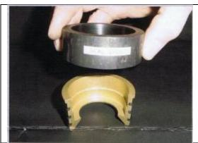
Step 1 – Apply light film of lubricant to inserts or housing I.D. to facilitate assembly. Place counter bore side of seal guide down onto housing as shown.
