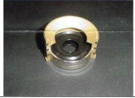
Step 6 – Pack area between the two inserts with a low-melting point grease. Add proper 0-rings. Part is ready tube installation.
